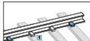
Remove clips attaching rails to sleepers on either side of the point to be cut.
