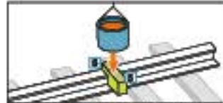
Build mould. Seal mould using gas torch. Drop weld into mould. Wear protective goggles and gloves.
